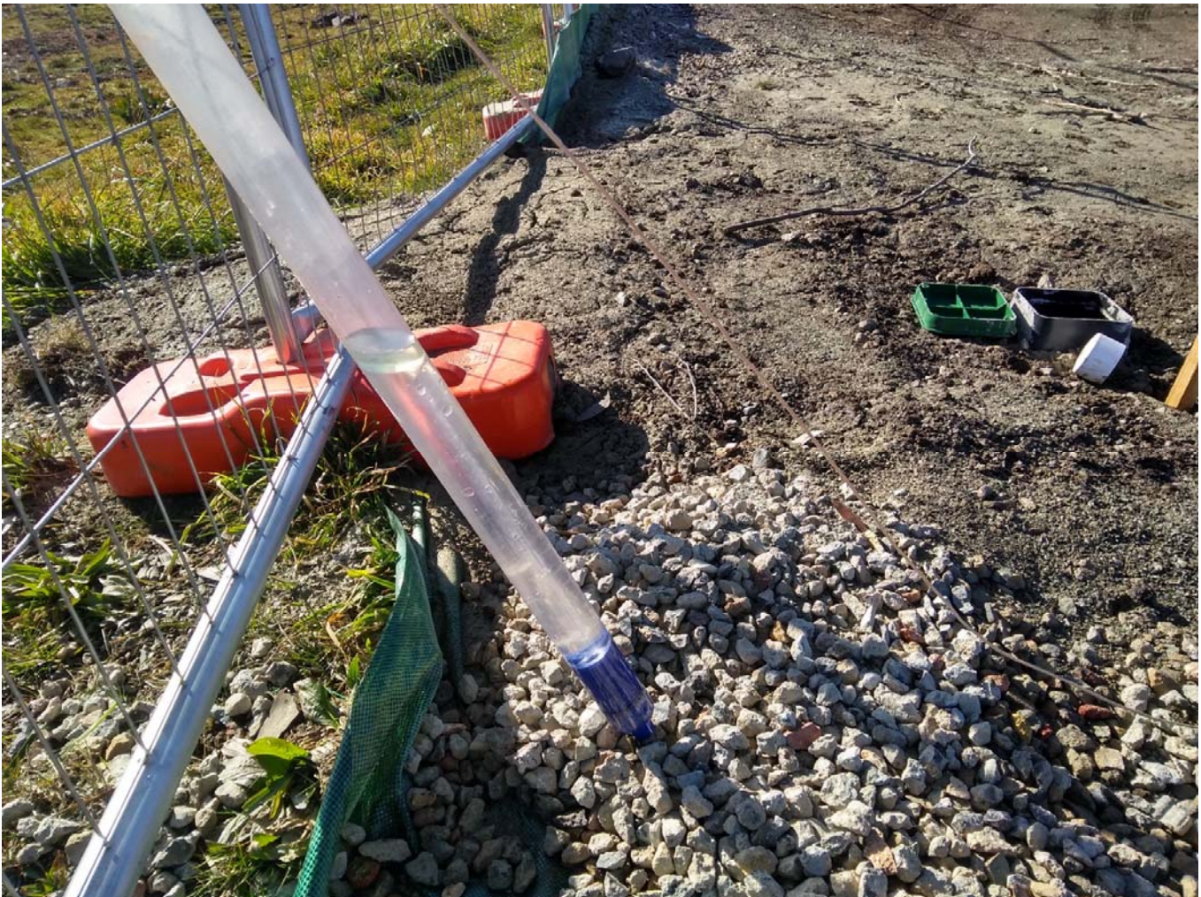
A small amount of LNAPL (diesel) was identified on the surface of groundwater within MW2.
